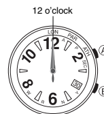
Correct hour and minute hand home position
